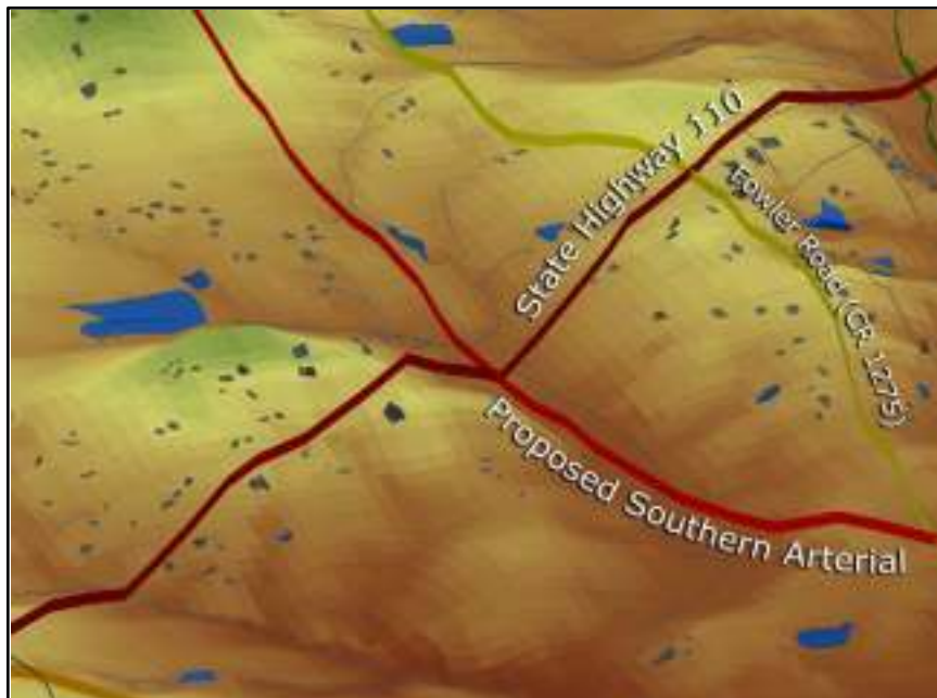
Image 11.3: Topography will play a major role in the final alignment of proposed thoroughfares. In this exaggerated elevation rendering (exaggerated by a factor of seven) the topographical concerns faced in southern Whitehouse are shown as they relate to the proposed southern arterial. Unfortunately the proposed route may be the only viable option for this connection that does not require the use of eminent domain to acquire right-of-way through land with pre-existing development.
