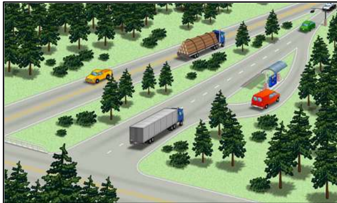
Image 7.8: Proposed on-ramp design for Loop 49 using TxTag automated toll gates (Image Source: Loop 49 Project Website)
